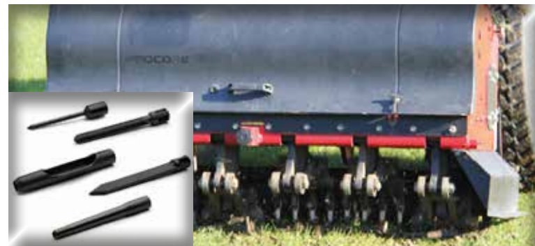
Bayonet or solid tines are a great alternative to core aeration, are less disruptive and play can resume quicker.
