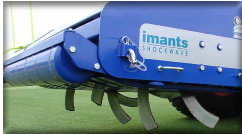
Linear decompaction up to 10 inches deep
